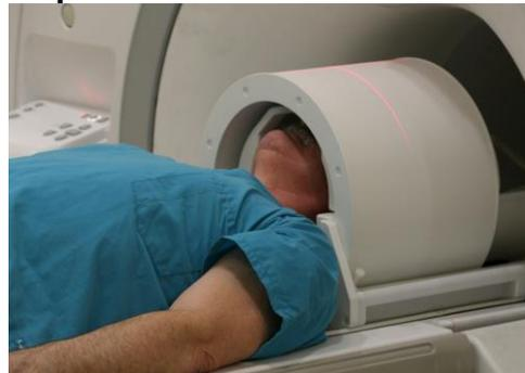
Typical use of the coils would be to use the volume coil for transmit and the array for receive. This provides maximal sensitivity and capability for accelerated parallel imaging. In this mode, all thirty-two array channels can be used for receive. However, the system can be used with the volume coil for both transmit and receive. This is useful for many applications such as shimming, scouting, and other operations which require a more uniform receive field.
