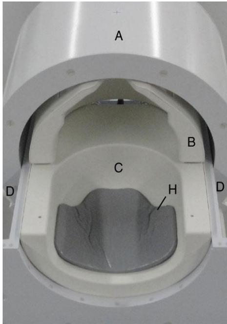
Volume Transmit, 32ch Array Coil
